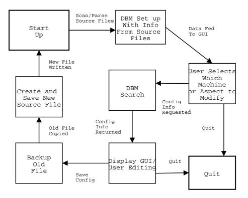
Figure 2.2: System Data Flow
