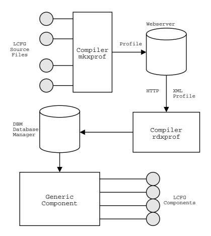
Figure 1.1: Overview Of LCFG Architecture
